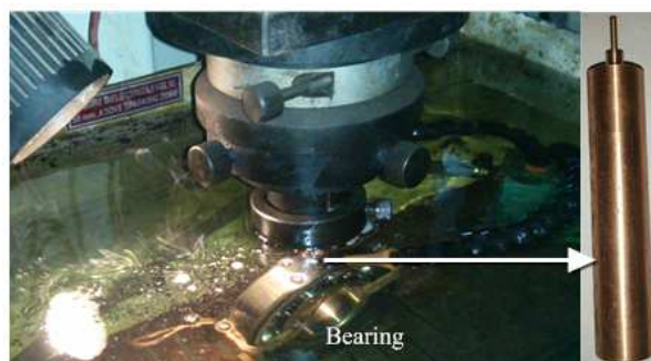
Figure 3.15: Electrical discharge machining underway for creating outer raceway fault and one of the sample copper electrodes used.
